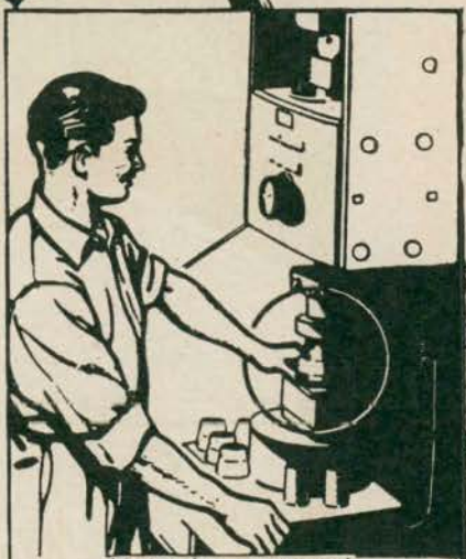
How tubes are tested To ensure the soundness of the weld, sections from every TRU-WEL tube are pressed over a cone in this special testing instrument.
