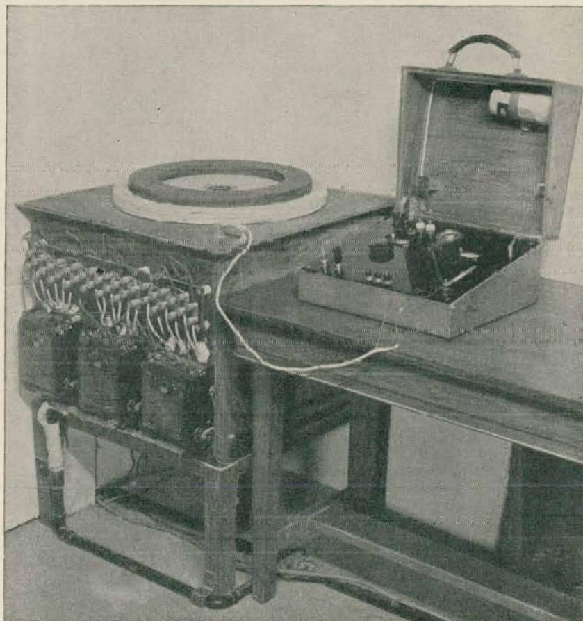
Fig. 1 A General View of Test Equipment Constructed at NPL for Testing Fire-Resisting Composition
